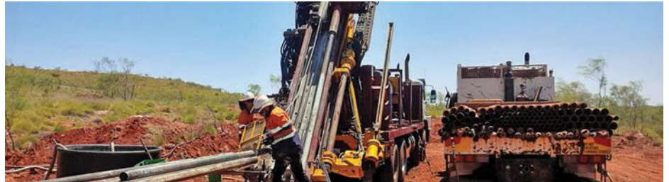
Geotechnical diamond drilling at Tabba Tabba in Western Australia
